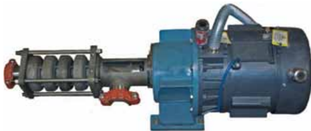
Figure 3. A four-stage, 300-gallon-per-minute, 500-psi pump by Fairbanks Morse with 6,600-rpm, 120-horsepower SR motor
